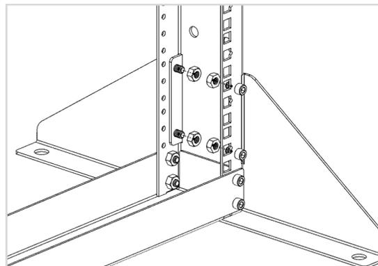
Assembly Tip: Hand tighten all bolts until the entire rack is assembled. Then go back and tighten them with the wrench.
